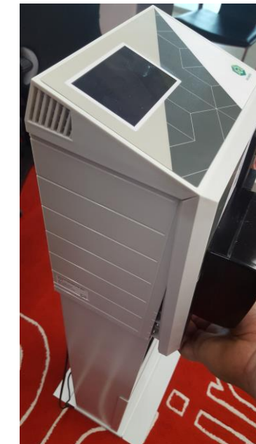
Step 5: Mount the SKUARIO Box on the pillar and close the front lid again
